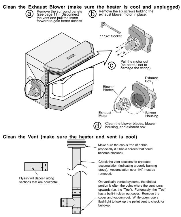
Warning: Whenever any portion of the pellet vent is disconnected, the joints must be sealed with RTV 500° F. silicone sealant.
